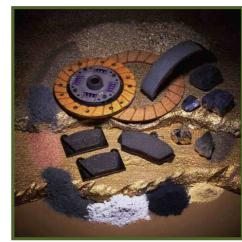
**LEAD SULPHIDE** (PbS) is typically used in the friction industry as a slip property modifier to improve heat conduction and regulate the friction coefficient.
